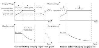
Lead-acid battery charging stages curve graph
